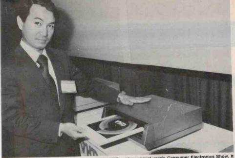
A Matsushita executive demonstrates the VHD system at last year's Consumer Electronics Show. It takes a vinyl disc that must be loaded with a caddle like the RCA system, but it has stereo (an add-on) and offers random access, freeze-frame etc.
