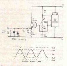
Figure 11. A 555 sine wave generator with a range of 83 Hz to 1.4 kHz (via R1).
