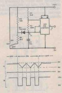
Figure 5. This slight modification of the C1 gating scheme produces a considerable change in the circuit output waveforms.
