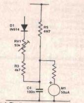
Figure 4. The linearising circuit. The meter is included for the sake of explanation. R4 replaces Link 1.
