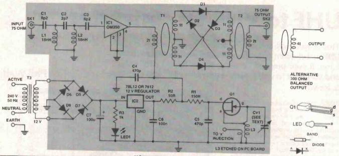
The converter's format is quite conventional — an RF amplifier drives a mixer, local oscillator injection being provided by a variable frequency oscillator, the frequency of which is set by a small variable capacitor. A full-wave bridge rectifier followed by a threeterminal regulator provides regulated 12 Vdc to power the circuitry.
