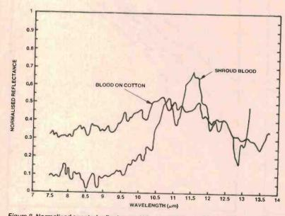
Figure 8. Normalised spectral reflectance of blood-on-cotton and Shroud blood in the 8 to 14  $\mu$ m infrared band. (Reproduced from reference 13.)
