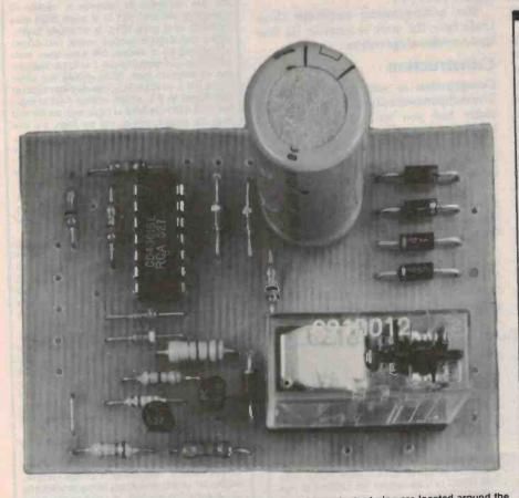
The relay driver board is simple, yet versatile. The external input/output pins are located around the edges of the board.
