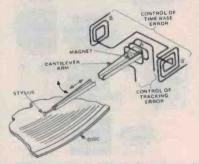
The VHD system from JVC employs a capacitive pickup system reading microscopic pits in the conductive plastic disc, tracking signals encoded on the disc providing information to a servo system that drives the stylus across the disc. Stylus life is said to be around four times that of the RCA system.
