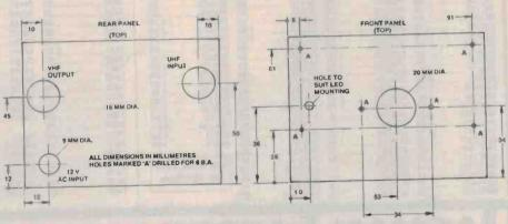
Panel drilling details for the Horwood box in which we housed the tuneable converter.
