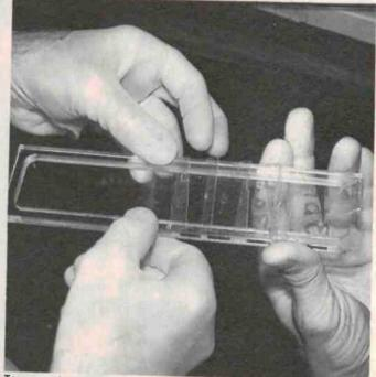
Tape samples taken from the surface of the Shroud are placed on specially sterillsed glass plates. (c) 1978 Barrie M. Schwortz
