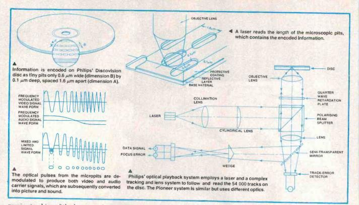
precise tracking of the laser spot beam together with servo control and time base correction to account for any warping of the disc. It is claimed that the laser modulated discs provide optimum picture resolution together with a long life, while the pits provide very high information storage density. The video blanking bandwidth can exceed 8 MHz. It seems likely that this system may offer sharper images than capacitive tracking systems.
