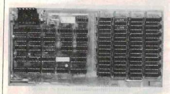
Unlike most other dynamic boards our's does not use the PSYNC, PWAIT, PHOLD, SM1, RESET, phi 2 and HALTA signals from the bus. Our board uses only one more control signal than most static boards. This means it is easier to interface to virtually any system. We have extensively tested our dynamic board with the DGZ80, Base 2, Jade, Cromenco and SD100 CPU cards. The TCT dynamic board is being used with Versafloppy, Micropolis and Tarbell floppy disk controllers.
