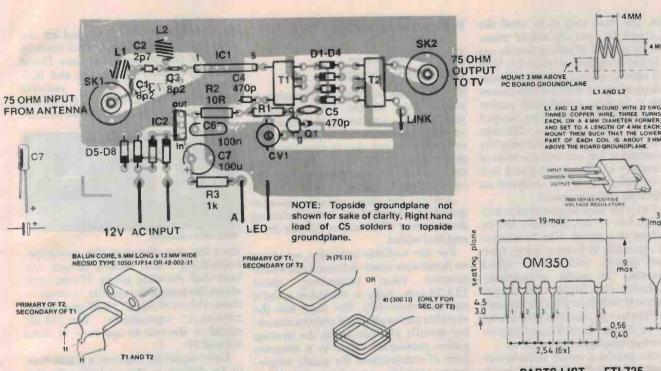
former. Overall gain is around 12 dB and the noise figure is around 6-7 dB. This sort of performance is more than adequate for normal service reception of UHF transmissions.
