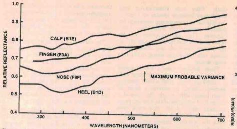
Figure 3. Relative spectral reflectance of four regions of the body image. (Reproduced from reference 12.)
