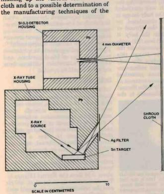
Figure 1. The apparatus used for the X-ray work. (Reproduced from reference 11).
