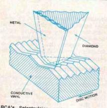
RCA's Selectavision system uses a metaldiamond composite stylus running in modulated grooves on the disc. The stylus tip is only 5  $\mu$ m by 2  $\mu$ m and the groove pitch is 2.6  $\mu$ m. Wear is said to be its biggest problem.
