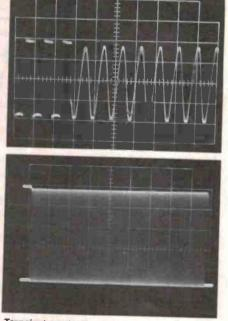
Transient overload recovery test (IHF-A-202) 1 ms/div 50 ms/div.
