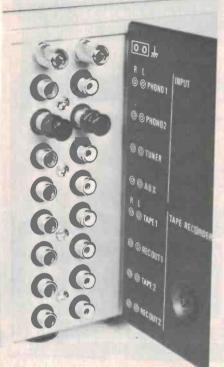
The input terminals are behind the front panel and go direct to the preamp pc board with minimum lead length. and found its performance superlative, particularly with moving coil cartridges and no less with moving magnet cartridges.
